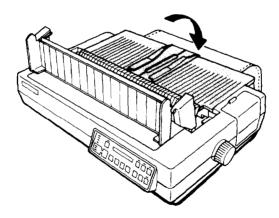
Note: The paper guide prevents outgoing continuous paper from being pulled back into the printer.
